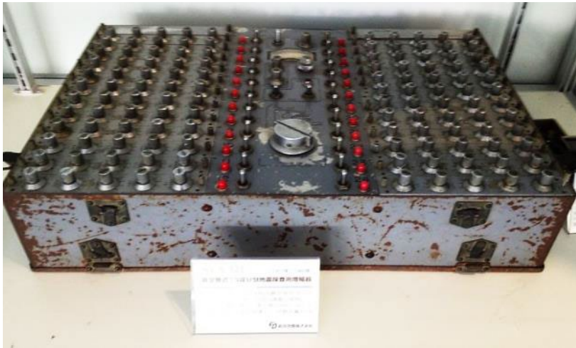
A vacuum tube type handcrafted from components purchased in Akihabara 13ch Seismic (ground strength structure) exploration device (in 1957)
